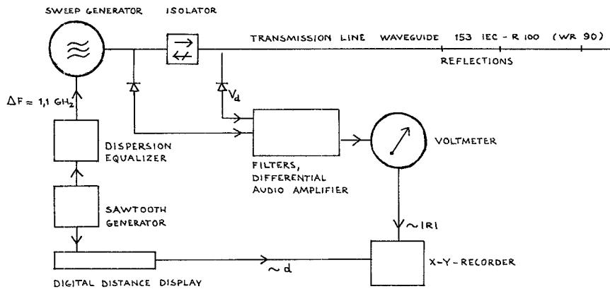
Fig. 1. Block diagram of the distance measuring system.
