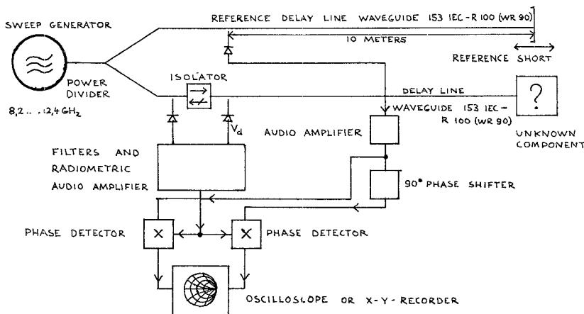
Fig. 2. Block diagram of the Smith chart plotter.
